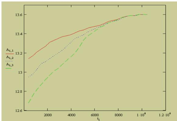
Oscilloscope graph of battery voltages during the Equalizing (Balancing) process: The voltages of the 3 batteries behave differently given the regulating influence of the BMLG<sup>®</sup> modules. The ideal harmonic charging curve will be achieved for every battery in the string.
