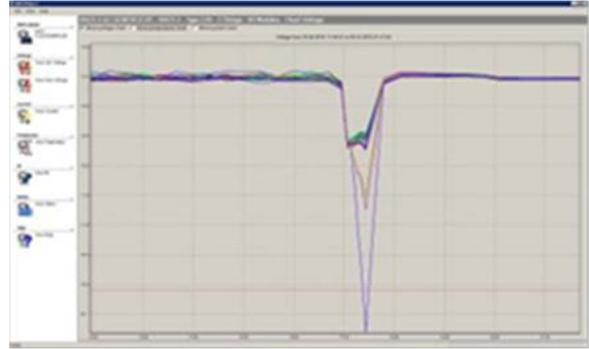
Discharge process displayed through BMLG® Viewer software shows the voltage drop of several batteries during a discharge, unnoticed by the UPS. In a later stage, these accumulators would cause the complete system to collapse! BMLG® corrects this problem and attempts to fully recharge this specific battery.
