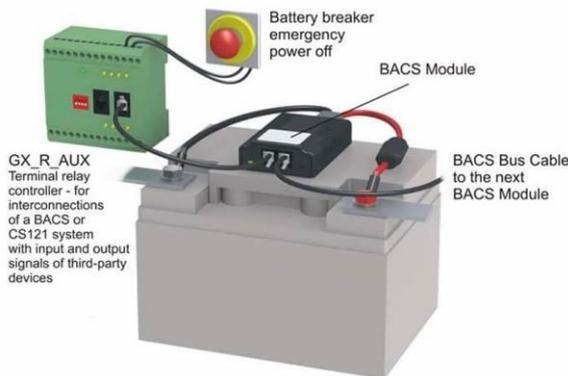
The GX\_R\_AUX module provides 4 relay contacts and 4 digital inputs. It controls up to 4 breakers. The digital inputs read the battery breaker status and display it in the BMLG® web interface. Other alarm devices (for example, audio alarms) may be connected to the outputs or digital inputs of the GX\_R\_AUX.
