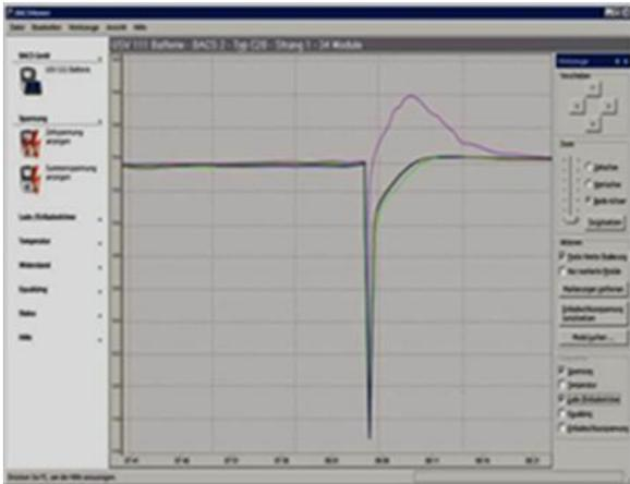
Free BMLG<sup>®</sup> viewer software shows the Equalization (Balancing) of a battery (the bold violet line in the graphic) within a string of 32 batteries during a discharge/recharging process. BMLG<sup>®</sup> Equalization (Balancing) prevents the overcharging of the violet battery, while the batteries around it continue to charge.
