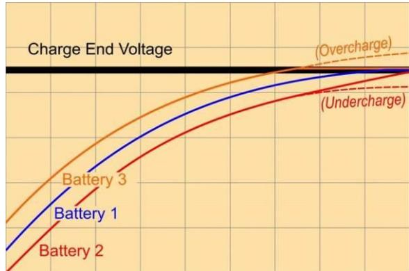
The charging of accumulators according to BACS<sup>®</sup> patented equalization process. The charging of Battery 3 is capped to prevent overcharging and gassing. Supply of charging energy to Battery 2 is continued and boosted until the target charging voltage is obtained. Battery 1 performs ideally and is not regulated.
