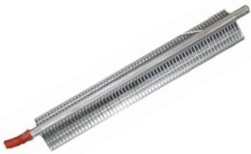
Electric heater consisting of finned aluminum elements, ensuring low surface temperature and deleting the air ionization problems. The optional is installed downstream the main cooling coil.
