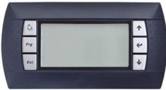
The microprocessor control system is equipped with 6 keys terminal and back lighted graphic display on which all information in different languages or easily identifiable symbols are displayed. The system disposes of a "flash" memory that preserves the information even in absence of power supply. Part of memory is dedicated to the registration of intervened events - up to 200 events.
