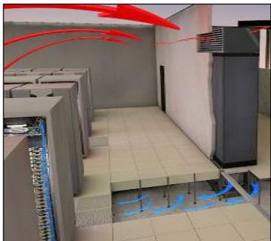
Some solutions provide a service corridor around the server rooms where to place the units. In this case, it is necessary to provide the air intake plenum for each unit. With this solution, all the space in the Data Center is available for the installation of racks.
