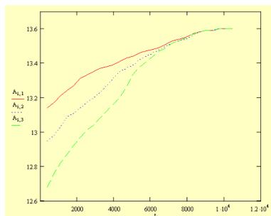
BLMG loading curves for 3 different charged batteries. BLMG takes care that all of the batteries reach homogenous voltage capacities after a short time.
